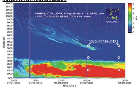
Volcanic ash identified using a Raymetrics LIDAR from the Eyjafjallajokull eruption in 2010 (data courtesy of NTUA)
