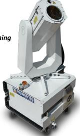
LIDAR Type: Raman, depol and/or backscatter LIDAR
