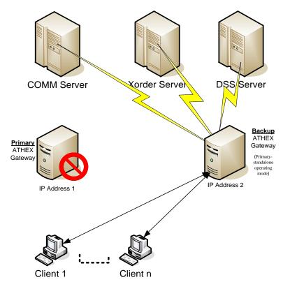
Figure 12-2: Primary – standalone ATHEX Gateway operation (after failover)
