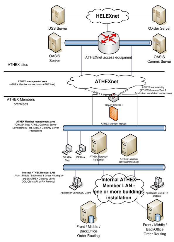
Figure 1-1 Equipment configuration required (hardware and applications) in the ATHEX Member sites and the ATHEX site for the ATHEX Gateway
