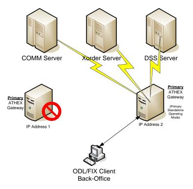
Figure 12-4: Double concurrent ATHEX Gateway operation (after failover)
