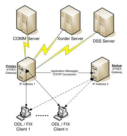
Figure 1-2: Primary – Backup Gateway configuration
