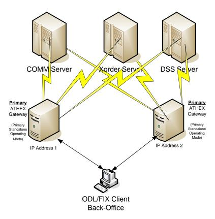
Figure 12-3: Double concurrent ATHEX Gateway operation
