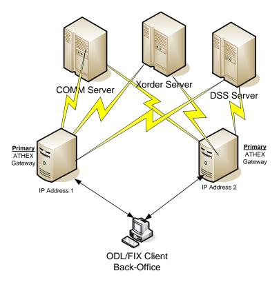
Figure 1-3 Double concurrent Gateway configuration
